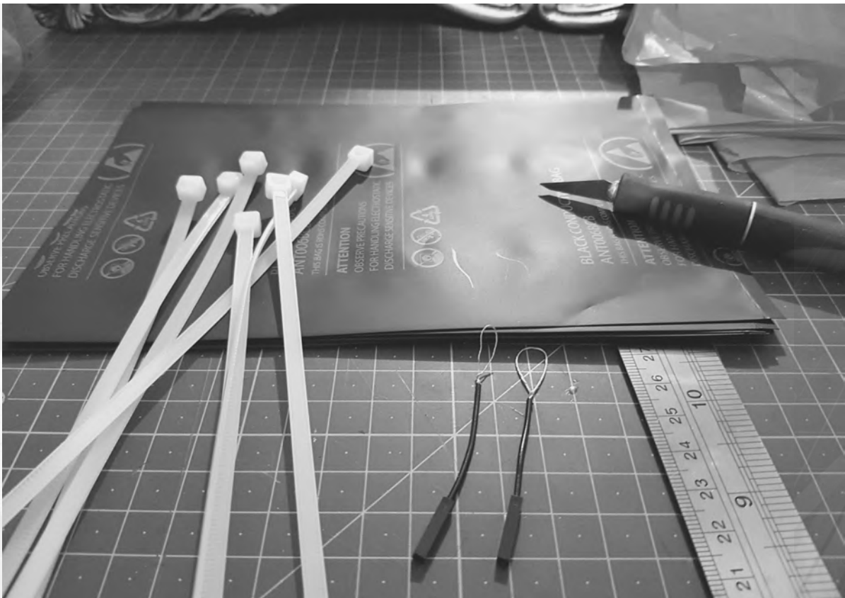
Figure 1. Materials used to create DIY flexible sensors.
