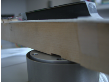
Figure 8: Setup with a K6D Force sensor for the piano key pressure sensor calibration. A black and white off-the-shelf piano key is used to calibrate the FSR sensors
