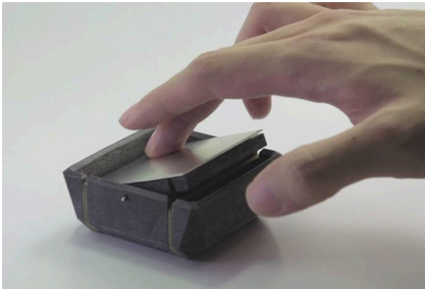
Figure 2. Pushing the touch plate sends aftertouch message useful for mapping to expressive variables.
