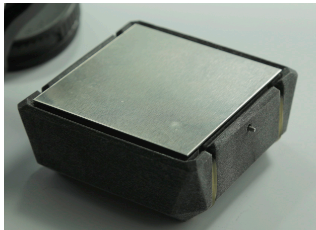
Figure 1. SoloTouch controller featuring a metal plate as capacitive sensor.
