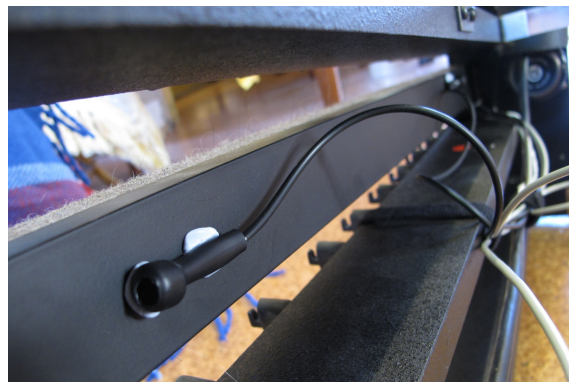
Figure 2: The microphones attached to the bottom of the damper bar.
