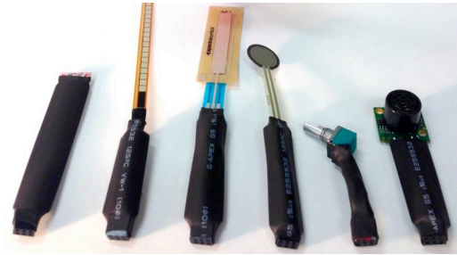
Figure 6: Sensor units (From the left: Infrared range sensor, Strain gauge sensor, Membrane potentiometer, FSR Pressure sensor, Rotary potentiometer, Ultrasonic Distance Sensor)
