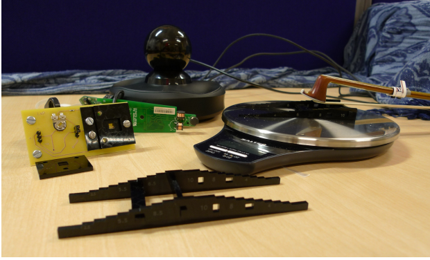
Figure 5: The various test tools (clockwise from rear)- the Razer Hydra and accompanying sensor, scale for future pressure tests with a height jig, height jig used for determining height lookup table, solder-free QRE1113 test jig for sensor evaluation.
