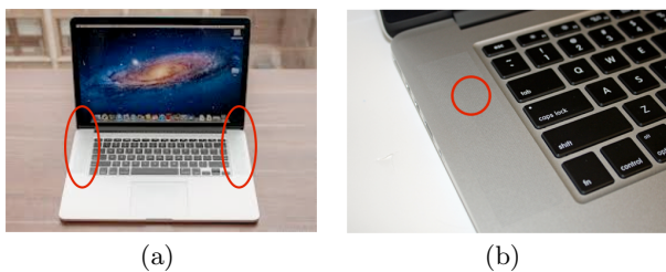
Figure 2: Position of the speakers and the microphone on MacBook Pro Retina. Two speakers are located on both ends of the laptop (a), while the microphone is only on the lefthand side (b).
