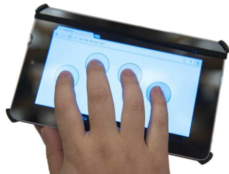
Figure 5: Multi-touch interaction with a Nexus tablet controlling sound synthesis on Satellite CCRMA via Interface.js .
