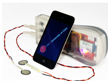
Figure 1: WLAN based sensor interface with 3D-printed casing.
