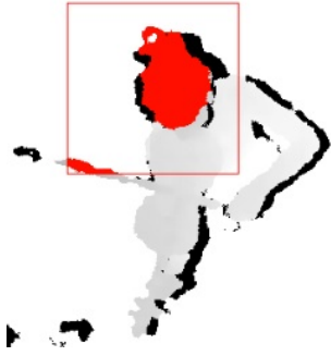
Figure 4: Head pixels are detected in a rectangular area around the highest head point based on the depth difference. Sometimes bow pixels are incorrectly labeled as head pixels.
