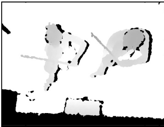
Figure 1: The raw image provided by the Kinect. Darker areas are closer to the camera; lighter areas are farther away. The heads and the bow tips are closest to the camera.
