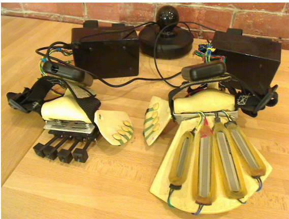
Figure 1: A complete Hand-Controller System with Track Platform, Slider Keys, boxed electronics, and the Razer Hydra
