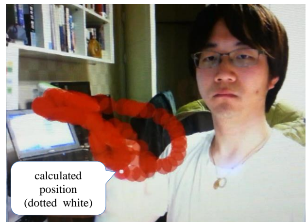
Figure 6. Virtual drawing by color recognition method
