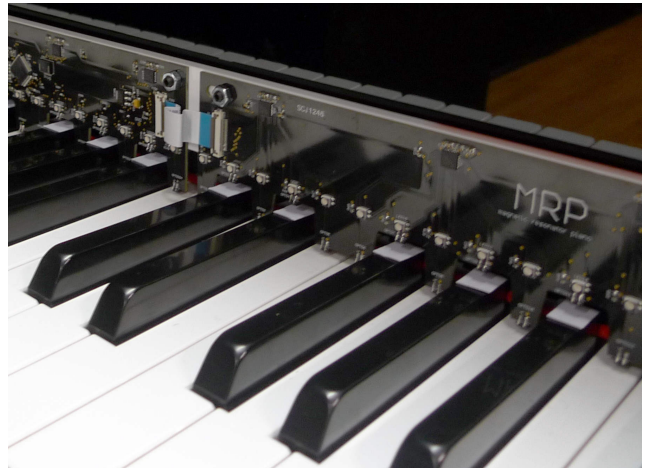
Figure 1: Optical scanner hardware. Top: scanner showing all RGB LEDs active, set up on the magnetic resonator piano. Bottom: optical sensors over each key. White stickers are attached to the black keys to increase their reflectance.
