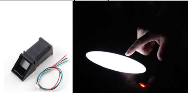
Figure 7. User input devices (a) fingerprint sensor ZFM-20, and (b) circular touch screen panel.
