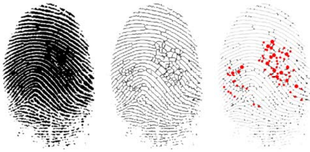
Figure 1. Extracted minutiae of fingerprints through image skeletonization and minutiae analysis.
