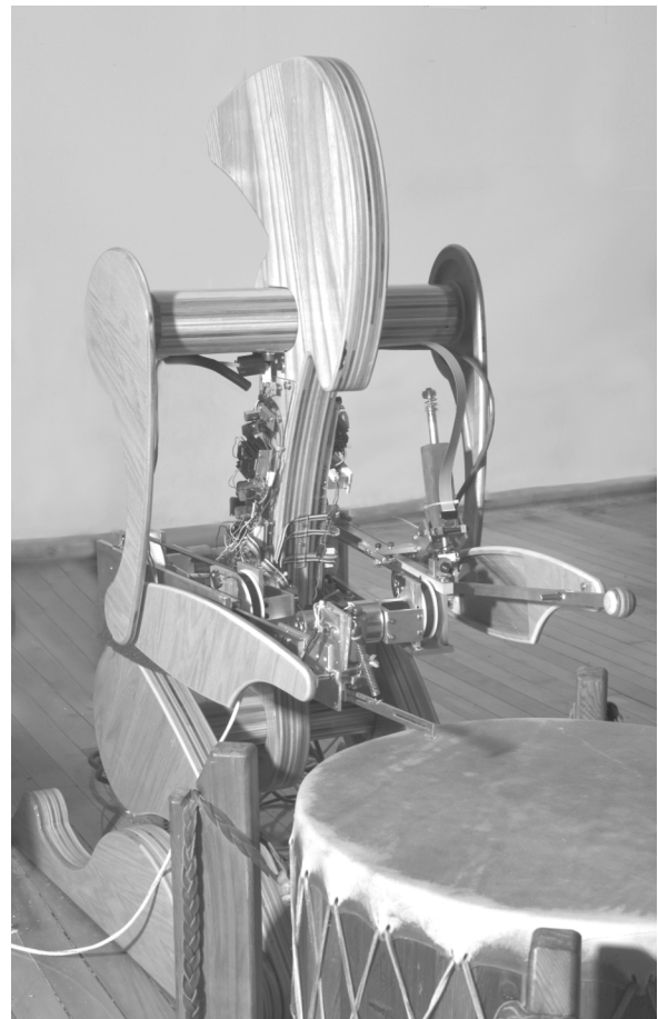
Figure 1: Haile - a perceptual robotic percussionist that listens and improvises with human drummers
