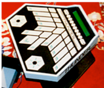
Figure 1: Thunder by Don Buchla. The ridge-separated strips are sensitive to both location and finger pressure. It sends MIDI controller data and is both continuous and polyphonic in character.
