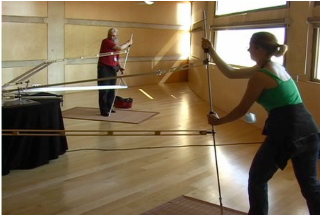
Figure 4. Frelia : an interactive kinetic sculpture; up to three users play Frelia by moving a 5-foot metal bar, whose movements are translated mechanically to the movements of a Wacom stylus on a tablet.
