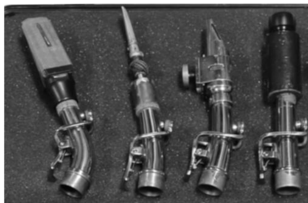
Figure 1. Different tone generators adapted for the soprano saxophone (from left to right): bawu-reed adapter, bassoon reed with adapter, regular saxophone mouthpiece (Otto Link, 13*), and an adapter for the cornett mouthpiece (C. Monk mouthpiece by Jeremy West).
