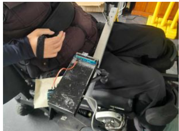
Figure 3. Analogue fader on bracket setup for time to target test – from above
