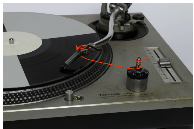
Figure 8: Tone arm with thread and anchor weight
