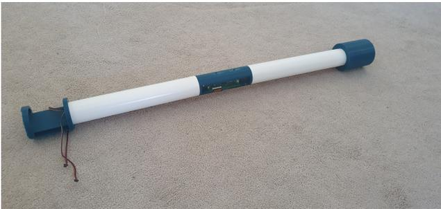
Figure 4: Partially assembled Soprano T-Stick 5GW. The touch board bed and endcap are glued onto the plastic pipe.
