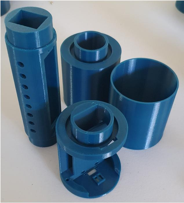
Figure 3: Components for the second version of the assembly, the touch board bed, and ESP32-S3 endcap are shown.
