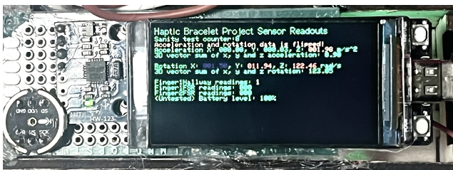
Figure 3: full-color TFT screen with realtime sensor readings
