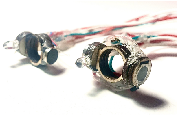
Figure 4: Laser cut rings with FSR, haptic actuator and LED
