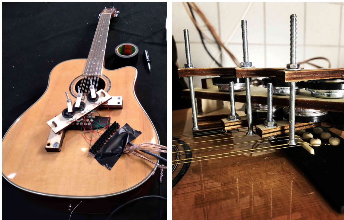
Fig. 2. Left panel: global view of a guitar with the excitation system mounted. Right panel: Closeup of the excitation system. Five electrodynamic transducers are glued onto a wooden board attached to the soundboard; one slat is glued onto the membrane of each transducer; a screw is attached to each slat and hits one string of a pair.
