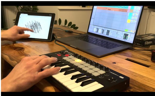
Figure 4: Setup using an iPad for sketch input that sends OSC messages to a Max4Live patch to manipulate synthesised sound in Ableton Live for a demonstration that can be viewed at <https://youtu.be/4Yzv2rgTg0E>.
