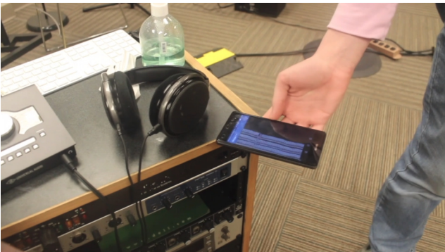
Figure 5: The Huawei P8 Lite running the MagSniffer to sonify the magnetic field generated by audio equipment.
