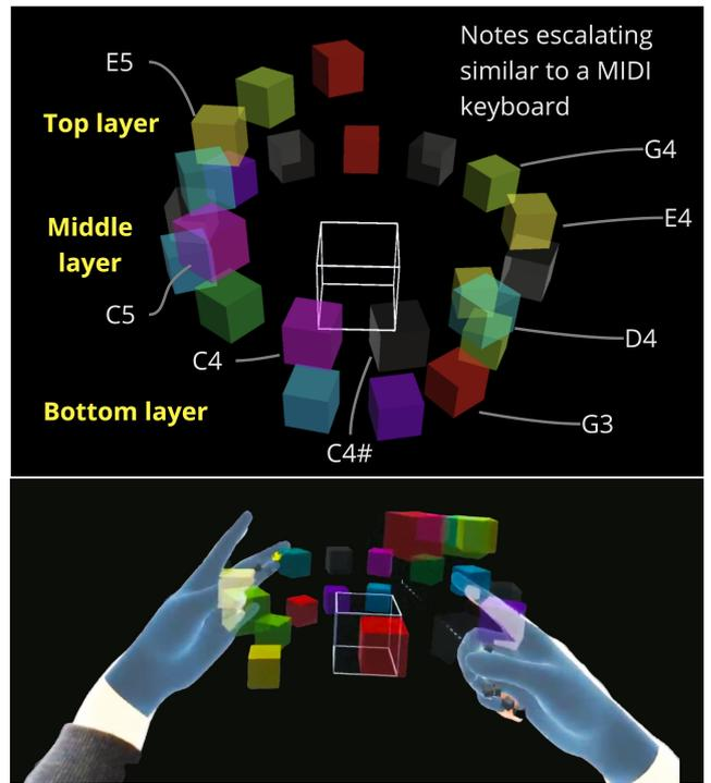
**Figure 2:** Top: the AR musical interface consists of three layers of coloured cubes and a cubic controller in the centre; touching each cube with a finger activates the corresponding tone. Bottom: an in-app view of the system in use.
