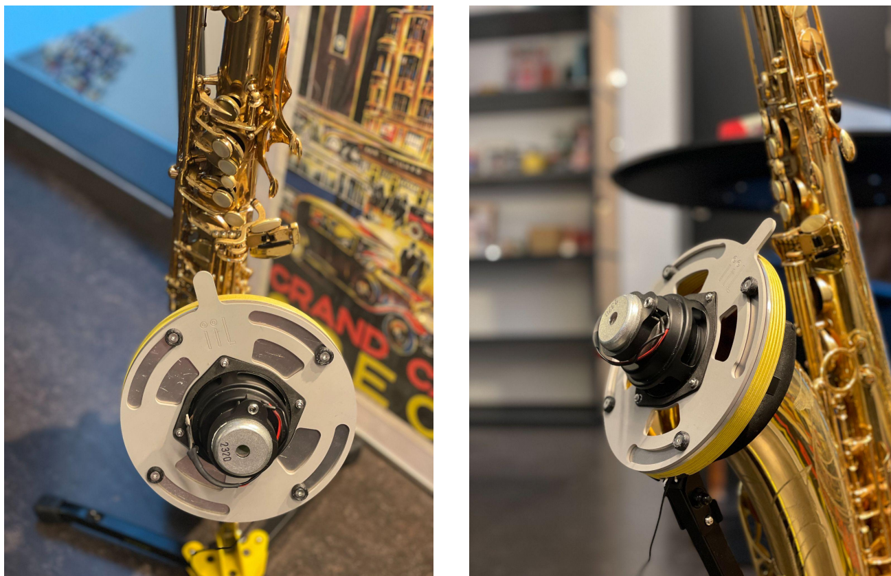
Fig. 1. Feedback saxophone with bell-mounted speaker and two-microphone configuration.
