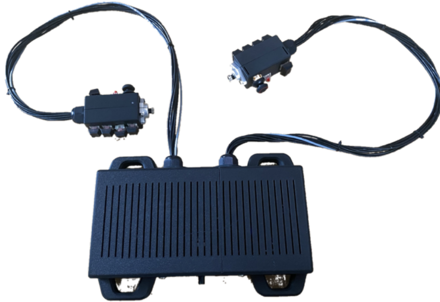
Fig. 4. 3D printed backpack and controllers. For wearing, straps are attached through the loops of the backpack.
