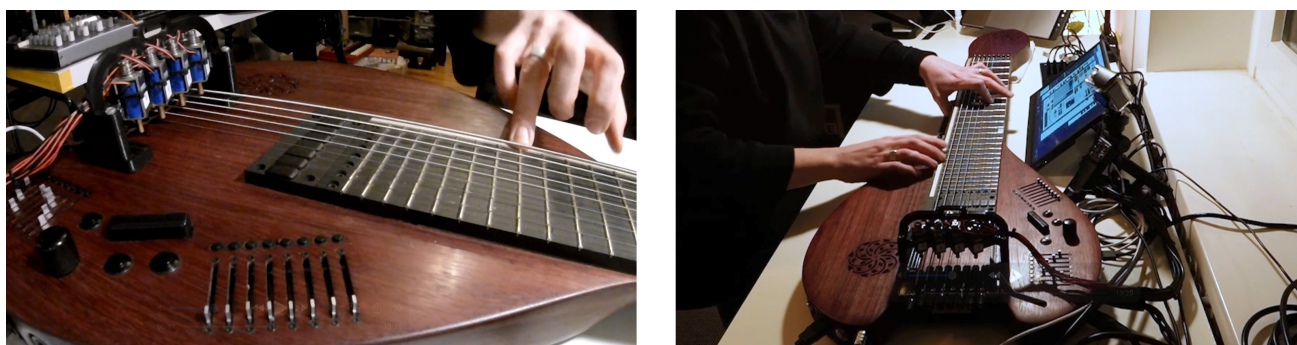
Fig. 1. The Sophtar's controls and actuators (left); the author playing the Sophtar (right).
