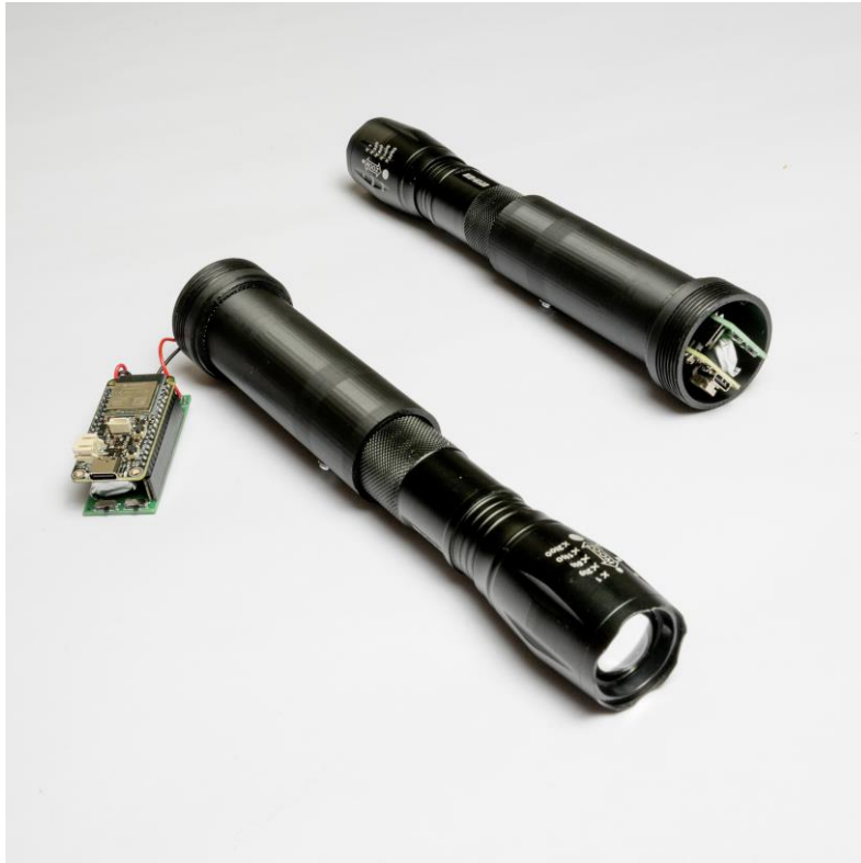
Fig. 6. Flashlights with their networked microcontrollers.
