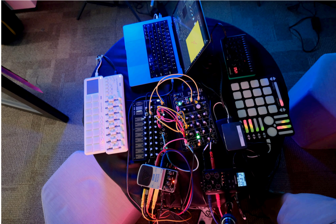
Fig. 2. The setup for our dual AI-feedback synthesis performance. Left: Make Noise 0-series synthesisers, laptop and Korg Nano series MIDI controllers, and an external reverb pedal is used as an optional effect during performance. Right: Raspberry Pi, Roland S-1 synthesiser and QuNeo controller.
