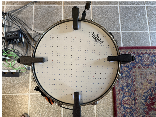
Fig. 1. Snare Drum with position markers for training neural network, 2025.
