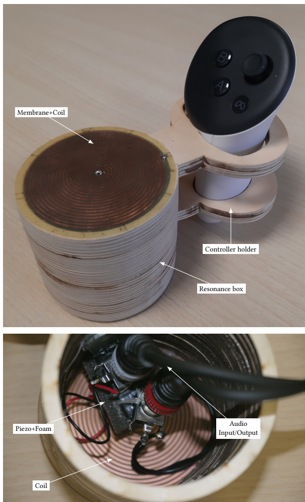
Figure 2: Initial instrument. Top: laser-cut resonance box and engraved membrane with coil. Bottom: connections to the coil as an audio output, and from the piezo pressed on the membrane as an audio input
