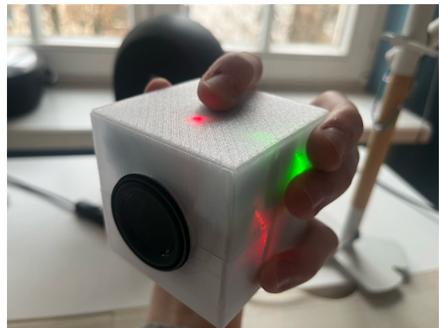
Figure 1: SonoCube held in hand, showing the 70mm translucent PETG enclosure and touch sensor LED indicator.
