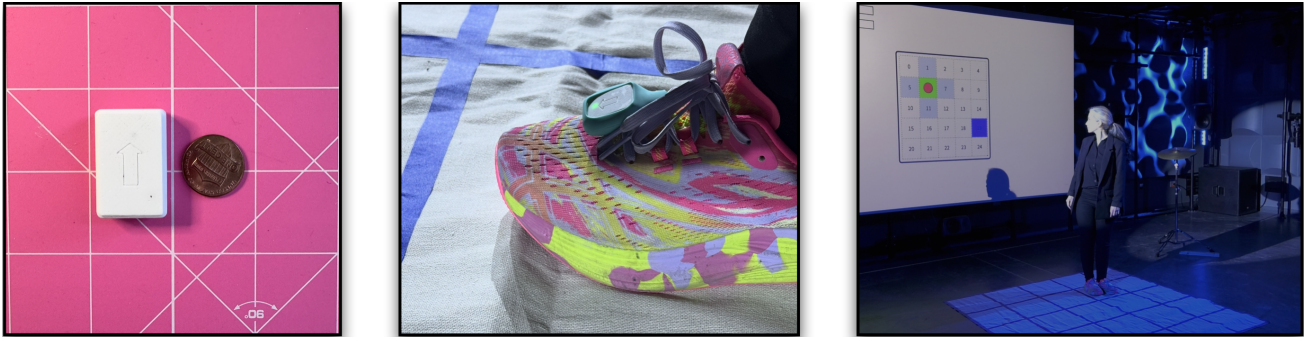
Figure 3: Left panel shows the battery and microcontroller with a quarter for size reference. Middle panel shows the battery and microcontroller wrapped into a module. The right panel shows the module embedded into a ball. Here, you can also see the opening that was cut into the ball.
