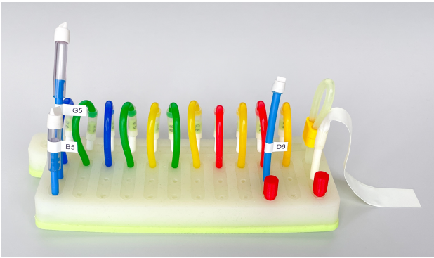
Figure 5: The pneumatic keyboard showing two modes for creating sustained sounds. Left: two whistles (G5 and B5) placed in the same column. Right: whistle (D6) and plug placed in the same column.
