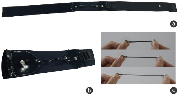
Figure 1: The breathing belt for respiratory measurement. (a) Overview of the belt assembly, featuring an embedded strain sensor at the center; (b) detailed close-up of the sensor placement; (c) visualization of sensor stretching across low, medium, and high resistance states.
