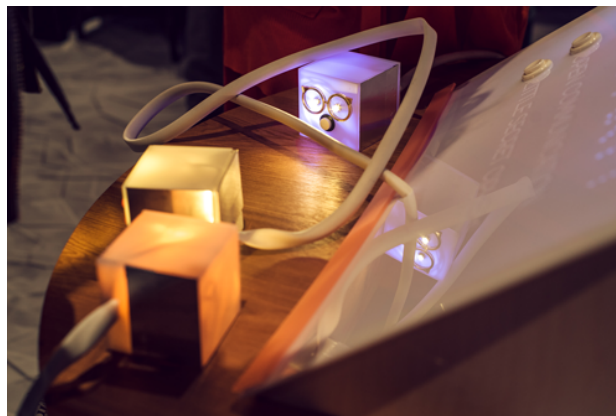
Figure 5: Bot Party Version 3: three LED-lit, transparent acrylic controllers in the arcade cabinet build.
