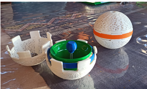
Figure 2: Two bell balls – the left ball is split open to reveal its tuned bell and weighted spring.
