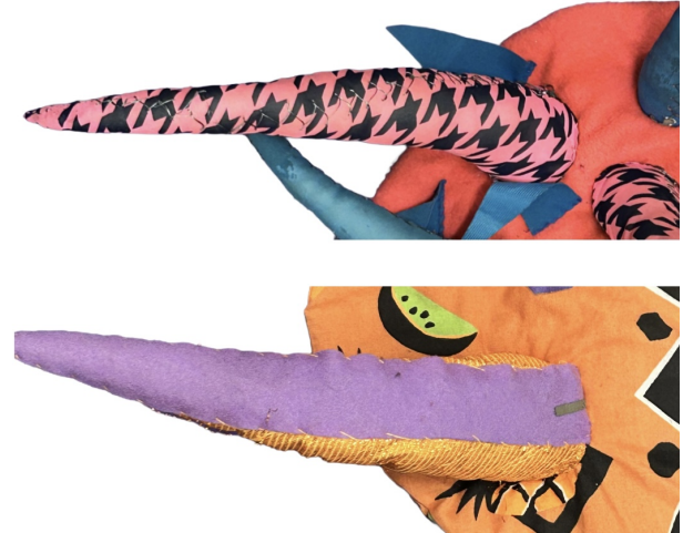
Figure 4: Top - V3 body conductivity input, updated with conductive thread, Bottom - V8 using a Velostat pressure sensor as input.
