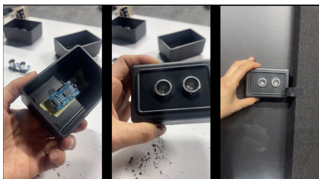
Figure 18: Boxes to place proximity sensors. Photos by Adriana Maria Gutiérrez Grisales
