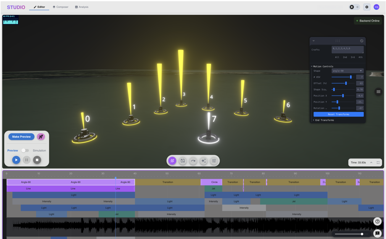
Figure 6: Parametric Motion Editor. Double-clicking the timeline (bottom) creates an effect, which can be dragged and resized. There are five effect types are Motion, Transition, Jet, Light and Intensity, which control movements and payloads. Upon selecting an effect, its parameters can be tweaked (floating panel). The 3D viewport (center) previews the choreography.
