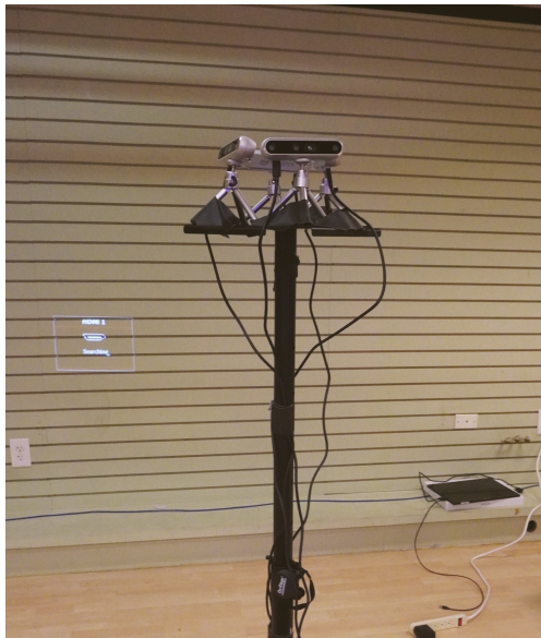
Figure 5: Camera-based audience tracking system setup.
