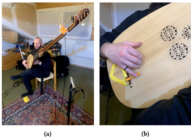
Figure 1: Theorbo devices: (a) the drone tuner installed with its pedal; and (b) the bender on the bridge.
