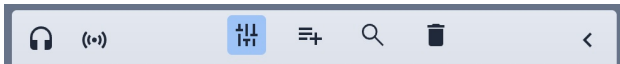
Figure 4: Headphone and Broadcast toggle buttons (left) allows one to turn on/off local and remote audio sending.
