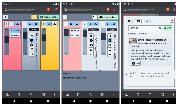
Figure 7: A pre-beta 2020 version of Mezcal with an extra yellow "call-in" track where producers have access to the mixing interface and listeners can only call in. Listeners and other producers could call in directly to one specific user if desired. This allowed ad-hoc configurations to be formed. The right shows a rudimentary search interface.
