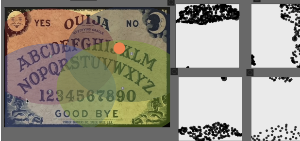
Figure 3: The Ouija patch’s node interpolation UI showing virtual locations of corpora audio samples are mapped to locations on the physical Ouija board.
