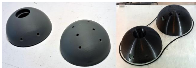
Figure 9: Body of the Ocarina printed in two halves on SLA (left) and FDM printers
