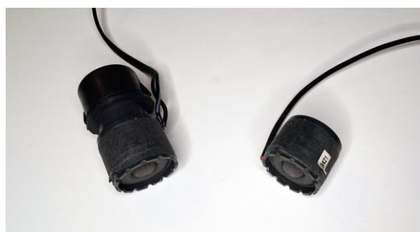
Figure 6: Original (left) and modified Monacor MD-110 microphone cartridge
