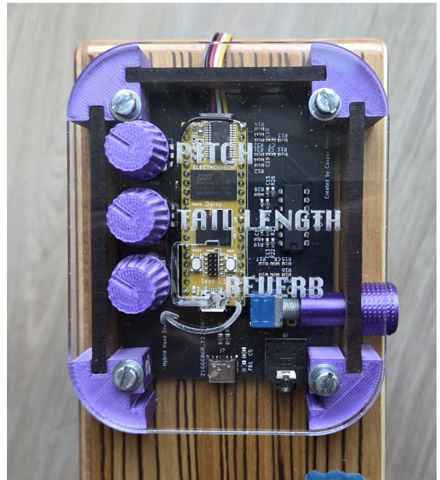
Figure 3: Iteration 1: user interface layout. Hole cut for mounting an ST-Link on the 10-pin header for flashing the Daisy Seed.
