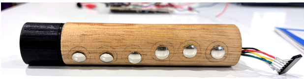
Figure 4: Detail of the capacitive touch sensors integrated into the carved wooden body.
