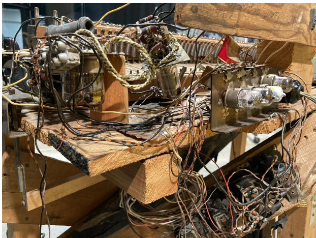
Figure 3: A close up of some of the circuitry inside the Electronic Sackbut, displaying some of the design and assembly style. The two leftmost tubes are the parent oscillator and a current source. The middle hanging tube assembly is the frequency divider board. The four tubes on the right in the center are the VCA. The transformers on the bottom right couple the VCA to the left hand joystick mixer, not shown. The discriminator circuitry, filter, and output stages are also not visible here. Photo by the author.
