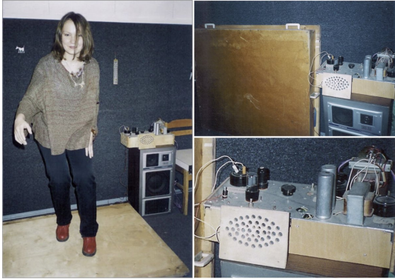
Figure 10: The photos of the Terpsitone, taken by Lydia Kavina at the Theremin Center in 2004. Left: Julia Koroleva shows position on the antenna panel. Upper right: the panel aligned with the wall nearby the tone block and a speaker. Lower right: the tone block and the speaker module close-up. Despite the drastic visual difference between this antenna panel and the one in Fig.9 - we confirmed, that this was the same device. The photo from 1982 shows it, covered with decorative fabrics, which were lost with time [15]. Photos taken from [28].
