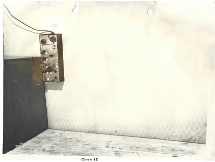
Figure 8: The Terpsitone from 1966-1968. We can see the segment of the floor panel (pitch control) on the bottom and the synthesizer module (tone block) mounted on the wall in a fashion of the studio Terpsitone from 1936. We can not confirm if the black panel on the left is a second antenna for the volume control. This most probably was the "small dance floor", described by Schonberg in New York Times. Primary source: [5].
