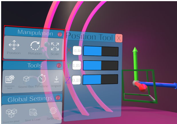
Figure 7: Illustration of the user interface used to modify the box transform. The interface is shown in position-editing mode.
