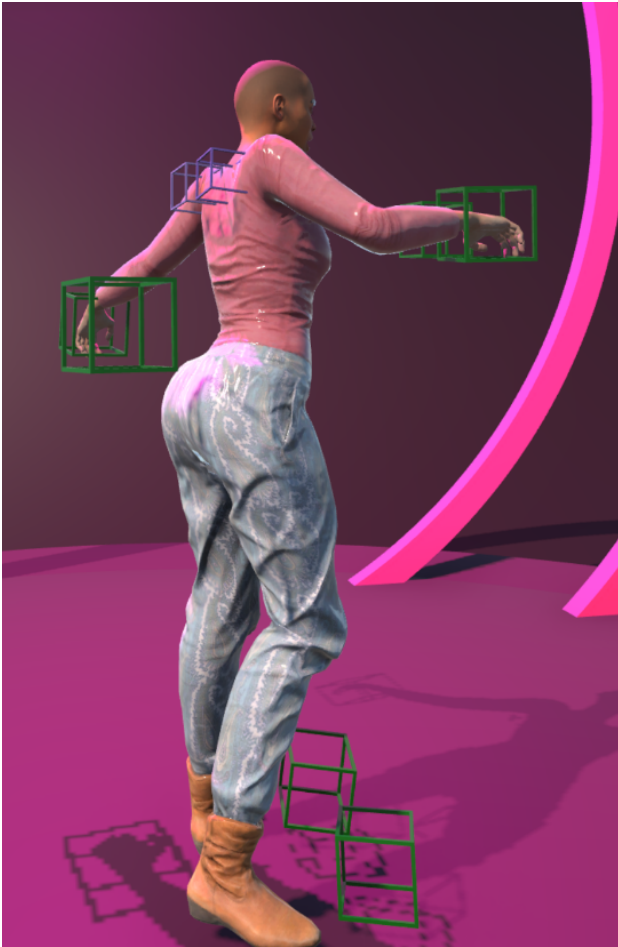
Figure 9: Box placement for large-amplitude, explosive movements: OSC boxes are positioned at the extremities of the movement to capture explosiveness, while EMG boxes placed on the trapezius record neck and arm muscle activity.
